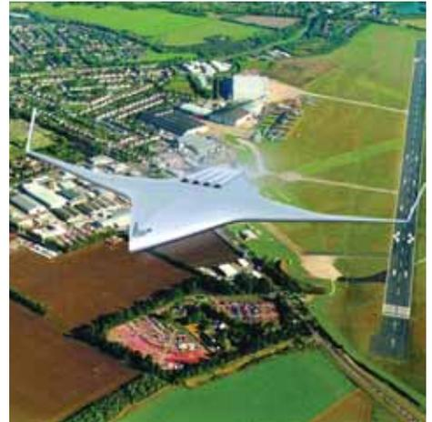
*Possible configuration of the Cambridge-MIT Institute's "silent" aircraft, which is expected to undergo extensive engine and airframe design for a radically different look, and sound, from current aircraft.*
