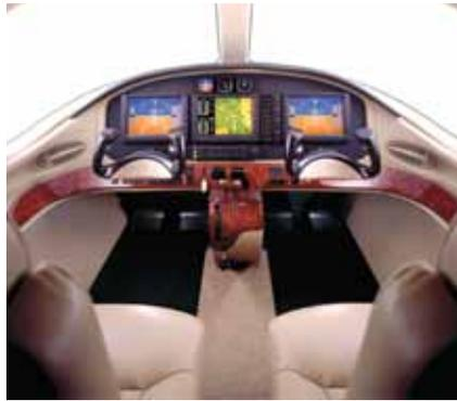
**The Citation Mustang will fly with Garmin's G1000 integrated avionics system that presents flight instrumentation, location, navigation, communication, and identification data via large-format LCD displays.**
