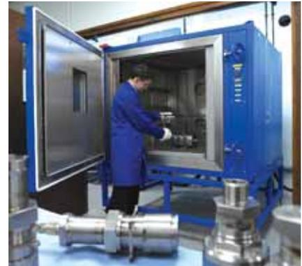
The internal chamber and door of the Carbolite chamber that FR-HiTEMP is using to test hydraulic systems for the A380 are fabricated from 304 stainless steel and are insulated to ensure safe outer case temperatures.
