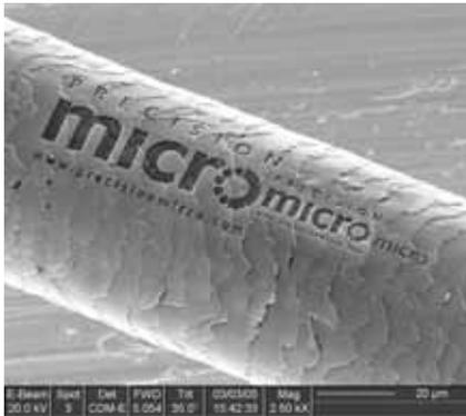
*Precision Micro and Birmingham University are collaborating on nanotechnology applications for the aerospace industry to take advantage of technologies such as focused ion beam systems, which are accurate enough to print logos on a human hair.*
