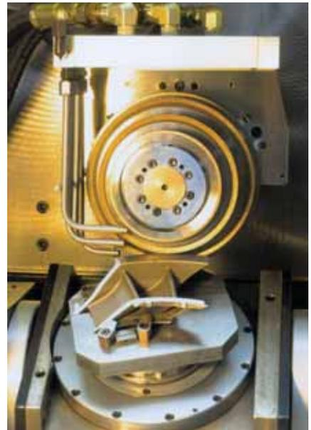
**Holroyd's Edgetek superabrasive grinding machine for the manufacture of jet engine compressor blades uses HEDG (high-efficiency deep-grinding) technology via high-speed cubic boron nitride, super-abrasive grinding wheels.**
