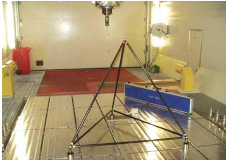
**metronom's Spatial Reference System (SRS) tetrahedron is in use by BAE Systems for the manufacture of elements of the Typhoon and F-35. The unique structural setup of the SRS bars is said to guarantee no dimensional influence in measurements through variation in humidity or temperature.**
