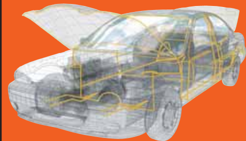
Structural bonding wireframe
